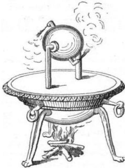
**Figure 1. Aeolipile Designed By Hero**
