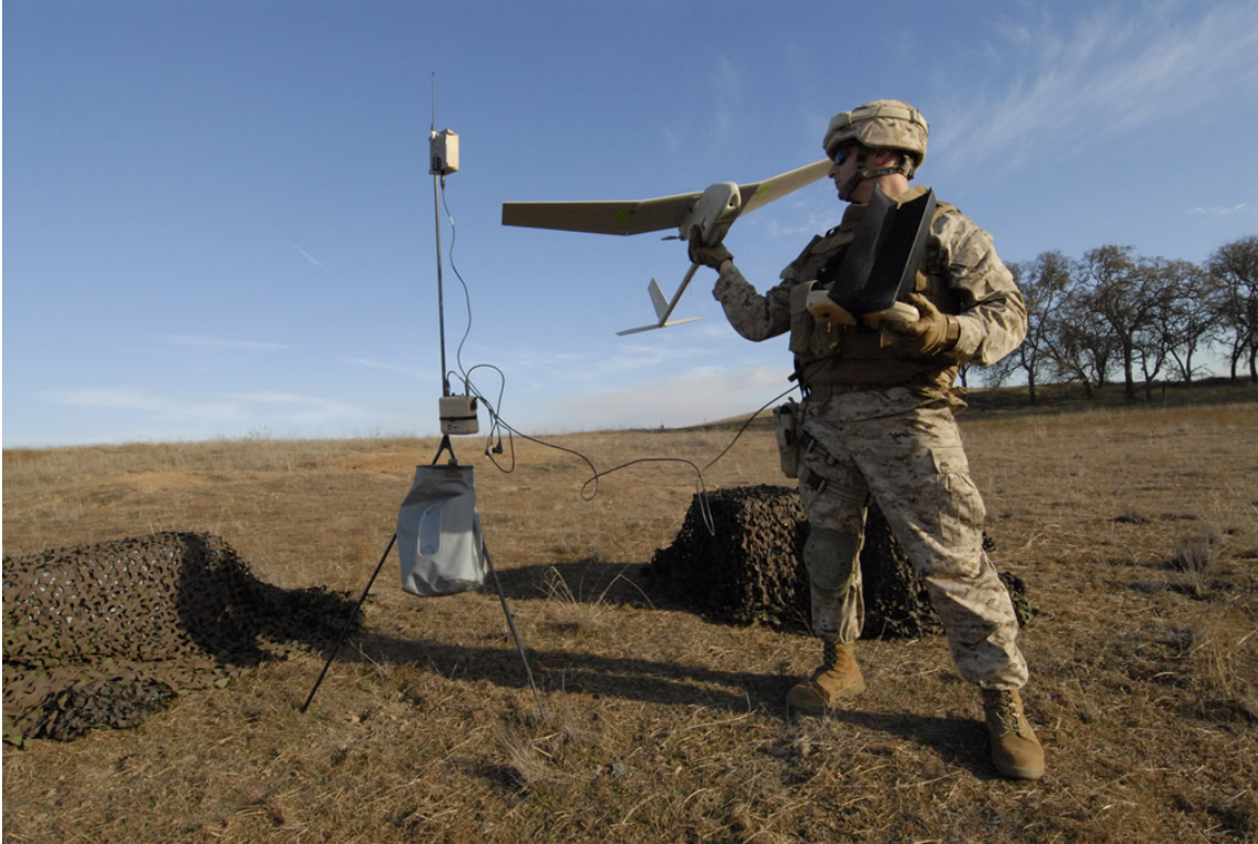
Figure 10. A Marine Hand-Launches the Raven UAS (AV, n.d.)
