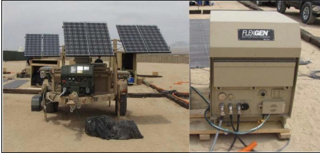
Figure 18. USMC Solar Stik MIL Series 3kW Trailer and Earl Energy 3kW FlexGen
