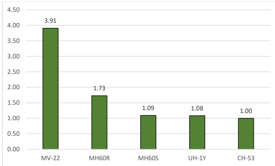
Figure 6. Ratio of Relief Radius by Aircraft Type
