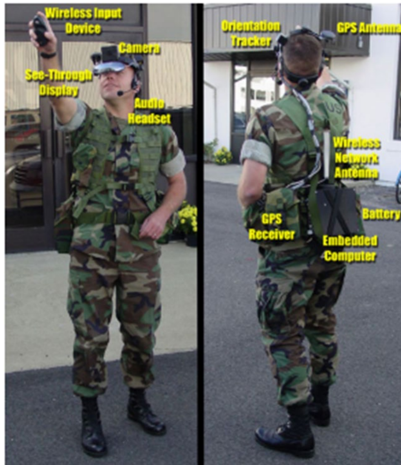
Figure 6. The Battlefield Augmented Reality System (BARS) Depicted with Each of the System Sub-Components. Source: Brown et al. (2005)
