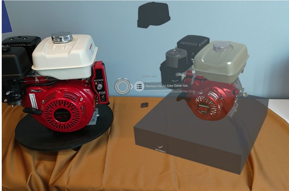
Figure 22. COACH System Displaying “the Orb” Task List. The Task List Directs the Removal of the Air Filter Cover Nut and Then Shows the Removal of the Air Filter Cover. Source: Redshred (2024).
