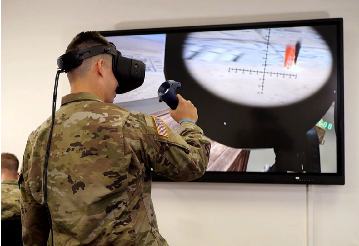
Figure 4. The JVT System Provides a Head-Mounted VR Device, a Set of Wands, and Software for Generating Immersive Training Scenarios for the User. Source: Xiphos Partners (n.d.)
