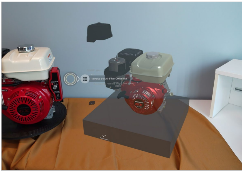
COACH system providing instruction to the user to conduct maintenance actions. Source: Redshred
