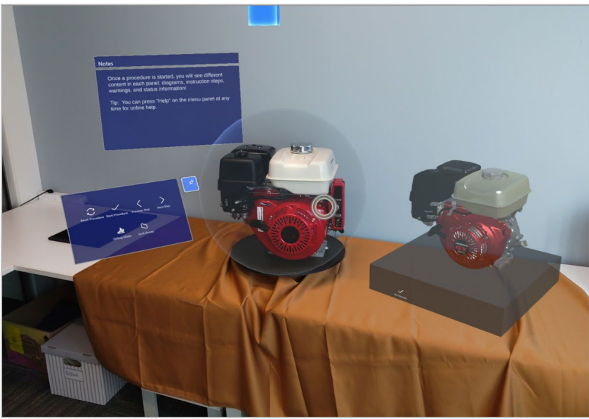
COACH system capturing the component that needs maintenance actions. Source: Redshred
