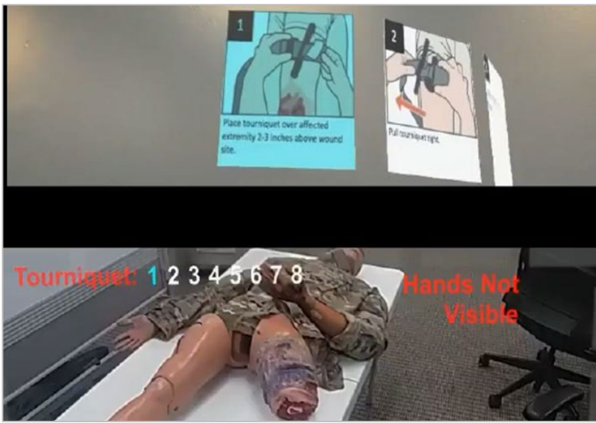
MAGIC system providing instructions to the user to apply a tourniquet. Source: Raytheon BBN
