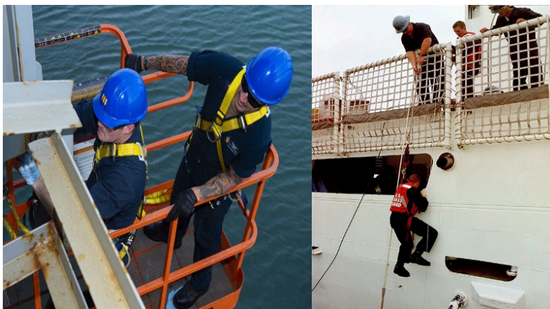
Figure 2. JLG Compared to Boatswain Ladder. Source: Dividshub.Net (2024).
