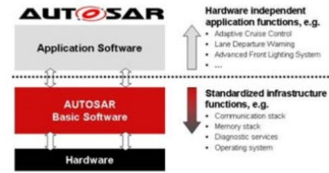
Figure 9. AUTOSAR Use and Structure. Source: Bunzel (2011)
