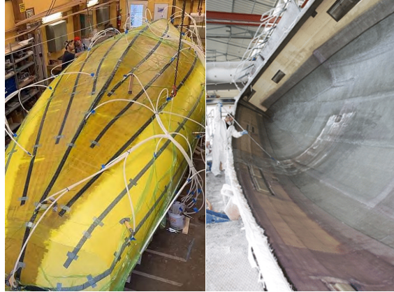
Figure 87. Vacuum Injection (Left) and Brush-On Fiberglass Molding. Sources: Artisan Boatworks (n.d.); Dufour Yachts (2016).
