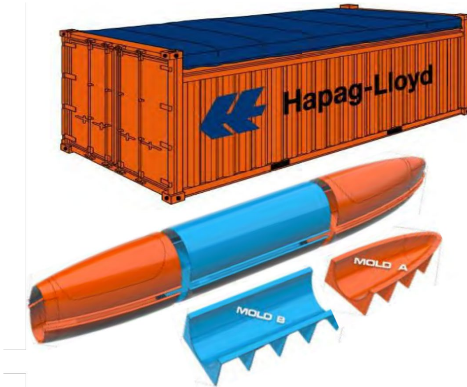
Figure 88. Modular Low-Profile Vessel, Mold Fabrication, and Container Transport. Source: Brutzman et al. (2024).
