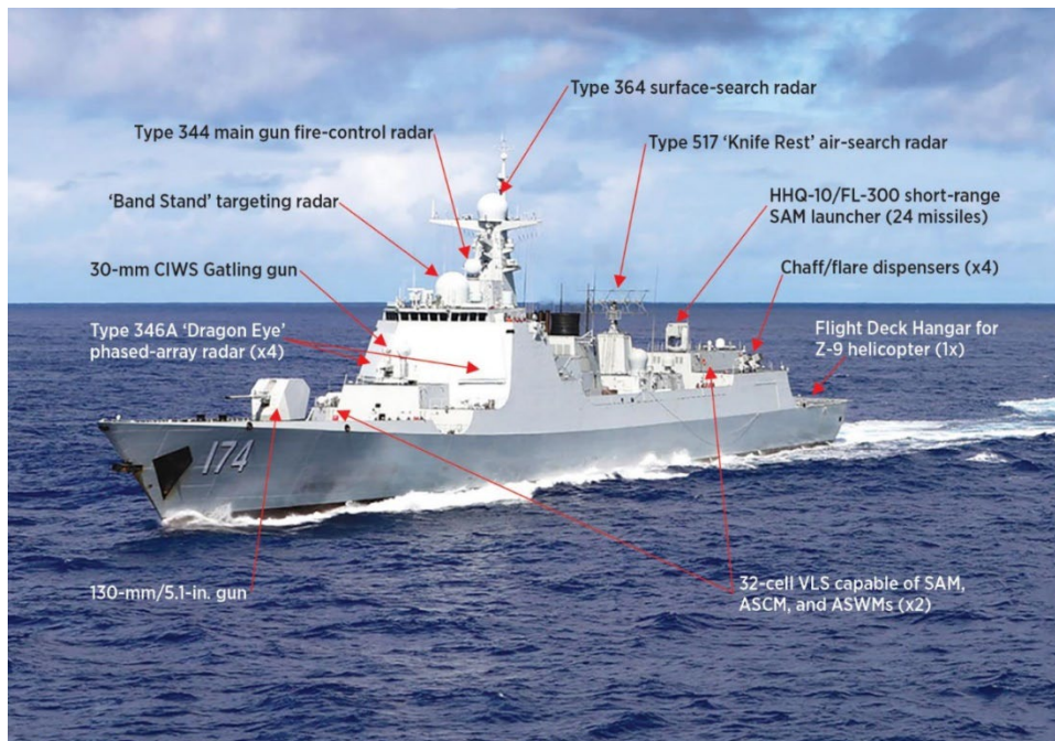
Figure 101. LuyangIII Class Destroyer Systems Callouts. Source: United States Naval Institute (2020).
