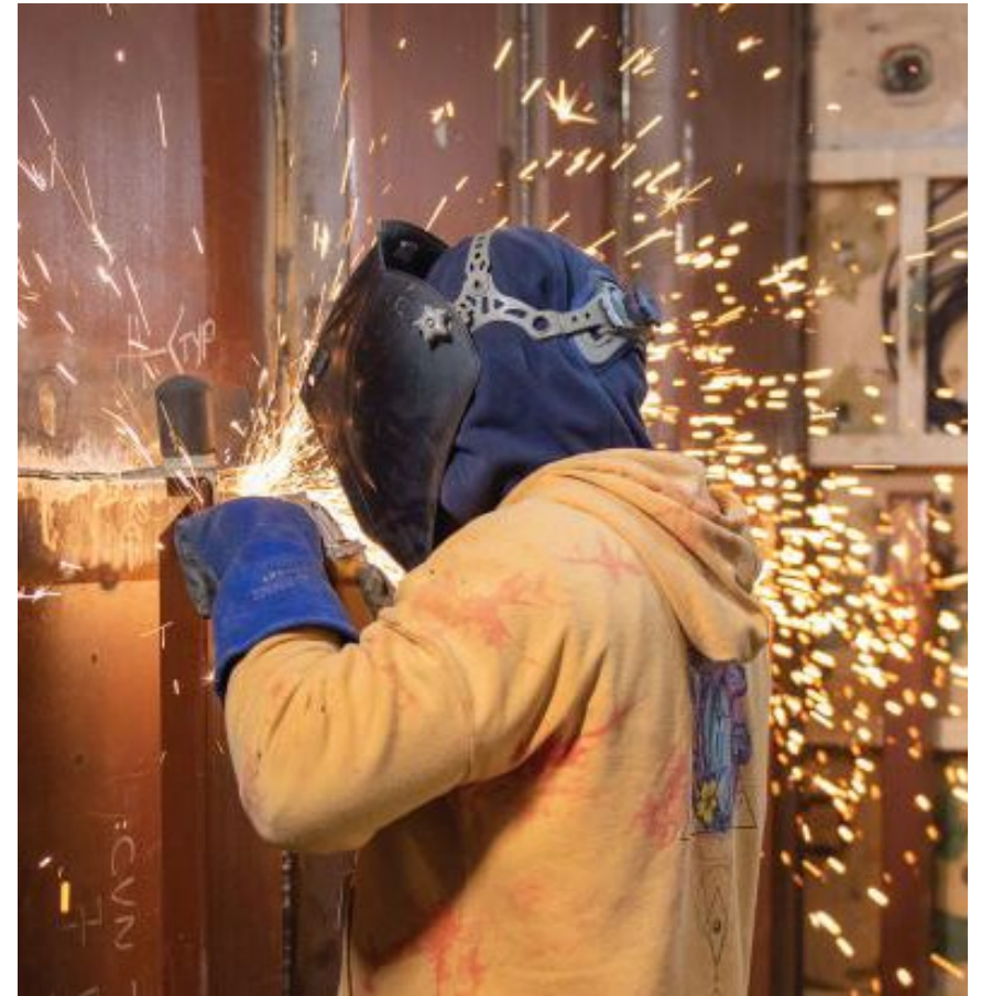
A Newport News Shipbuilding worker grinds on a camera foundation on board the aircraft carrier USS John C. Stennis (CVN-74). Image from USNI.
