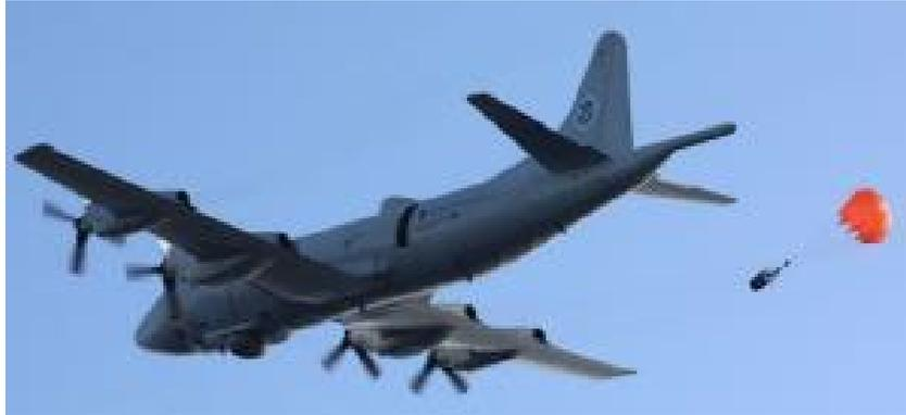
Figure 10. Airborne Deployable Delivery System. Source: Public Affairs CBP AMO (2024).
