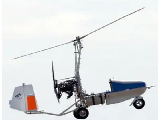
Figure 4. Gyrocopter UAV Configuration. Source: Szondy (2019).
