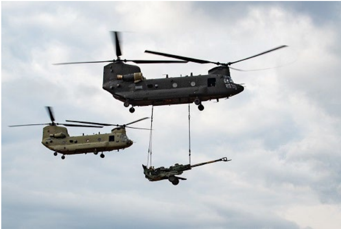
Figure 7. A U.S. Army CH-47F Block II Chinook Conducts a Sling Load Test. Source: U.S. Army Aviation Flight Test Directorate (2024).
