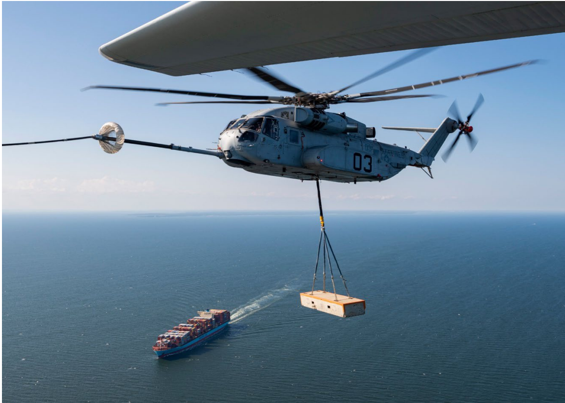
Figure 5. CH-53K Conducting an Aerial Refueling Test with an External Load. Source: Sikorsky (2020).
