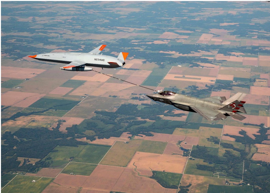
Figure 9. MQ-25 Stingray Conducting Aerial Refueling Testing of an F-35C. Source: Szondy (2021).
