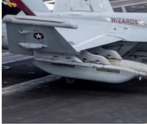
Figure 28. AN/ALQ-99 JTS Mounted on an E/A-18G. Source: Trevithick (2024).
