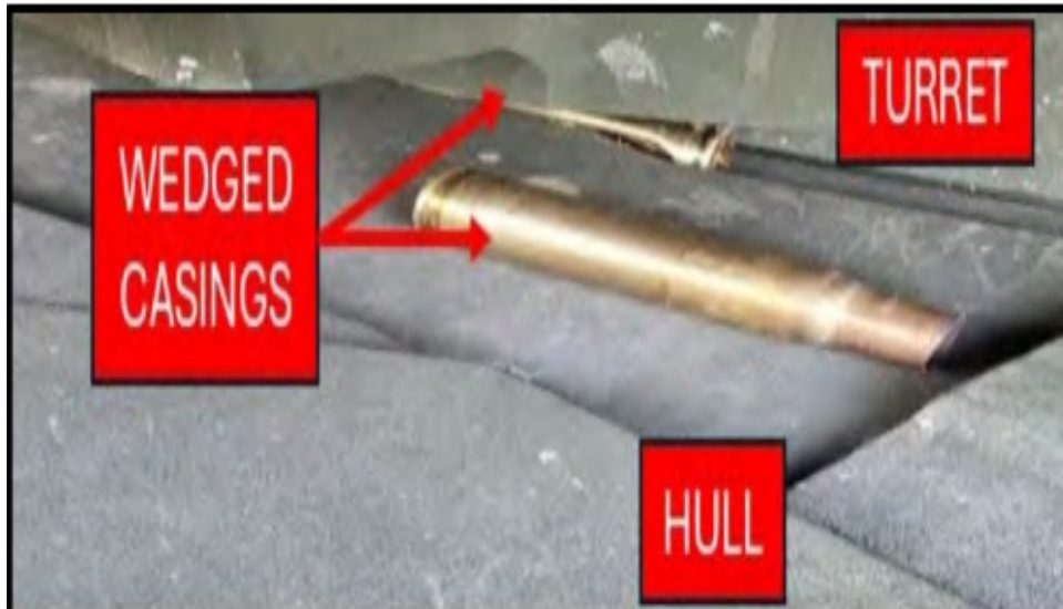
Figure 11. Casing Wedged between Turret and Hull
