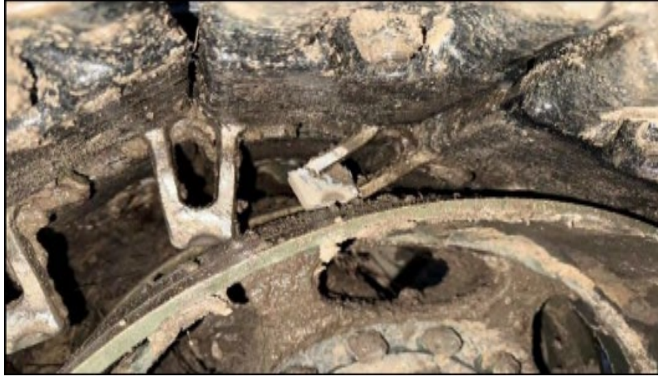
Figure 10. M10 Center Guide Damage
