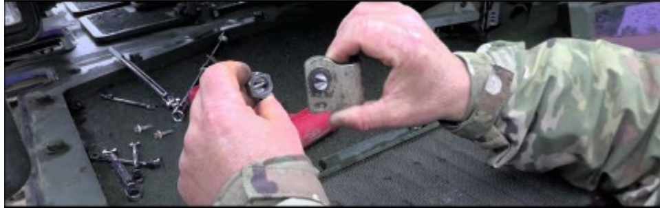
Figure 12. M10 Sheared Final Drive Bolt
