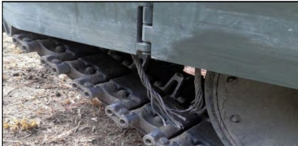
Figure 15. M10 Side Skirt Mesh Step Failure
