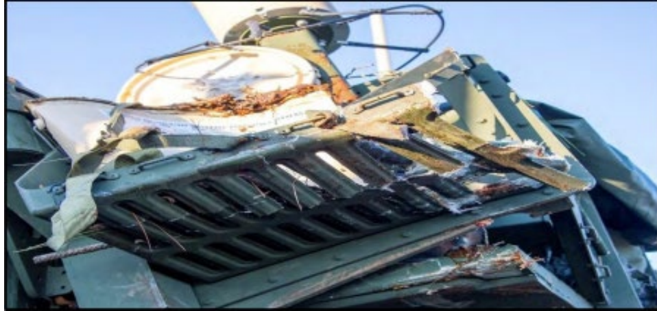
Figure 14. M10 Bustle Rack Damage
