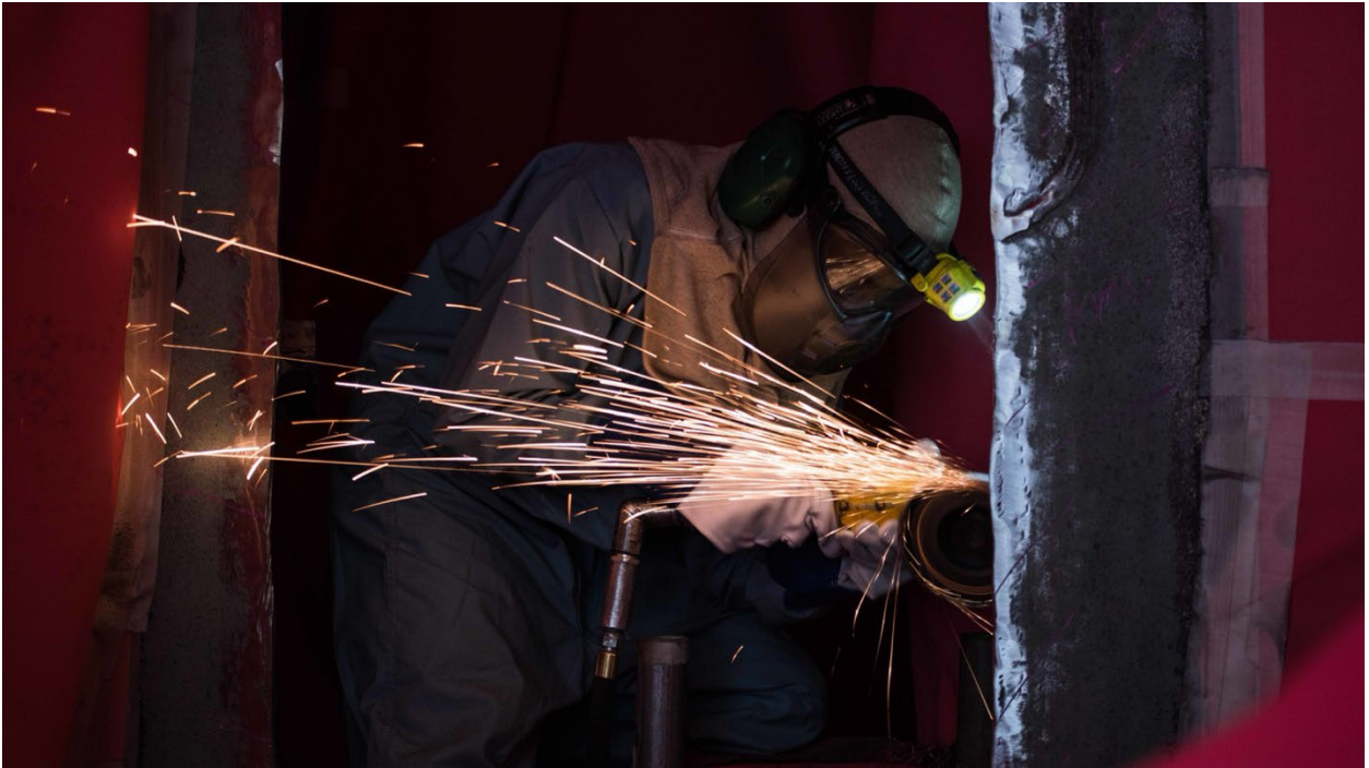
Figure 2. A Worker Grinds a Bulkhead at Puget Sound Naval Shipyard. Source: Kreishner (2019).
