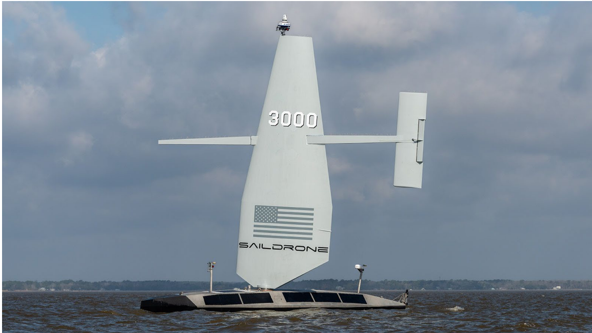
Figure 8. Saildrone Surveyor-class USV. Source: Saildrone (2024).
