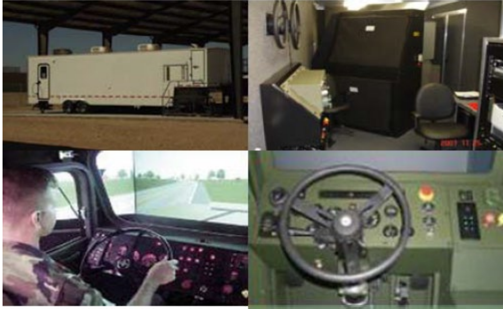
Figure 6. Operator Driver Simulator Housing, Cab, Display, and Dashboard. Source: Marine Requirements Oversight Council (2010).
